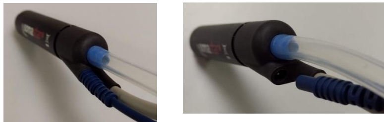
Figure 4.5: Monopolar Handswitch Handpiece Cable Connection
