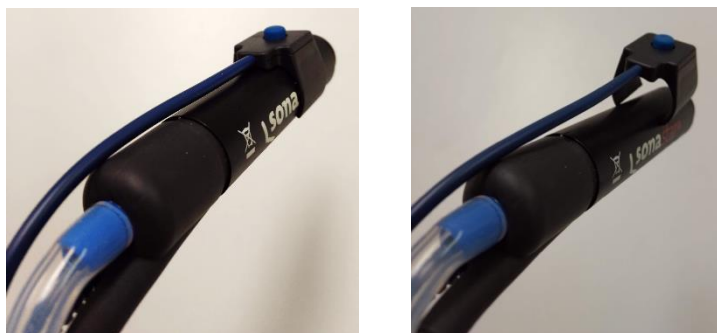
Figure 4.6: Monopolar Handswitch Housing Connection
