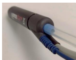
Figure 4.3: Monopolar Handswitch Handpiece Cable Connection
