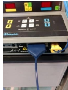
Figure 4.5: Monopolar Handswitch Electro-surgical Cable Connection
