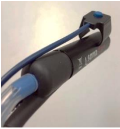
Figure 4.4: Monopolar Handswitch Housing Connection
