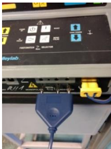
Figure 4.5: Monopolar Handswitch Electro-surgical Cable Connection
