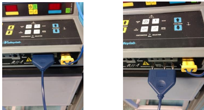
Figure 4.7: Monopolar Handswitch Electrocautery Cable Connection
